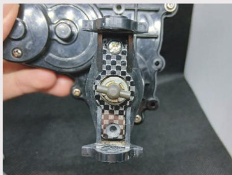
2) Drill through the lower hole with a 3mm drill bit.
