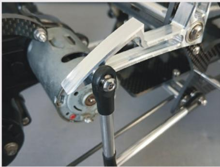
**2)** Fit the upper links to the chassis with the 16mm screws. Put a washer between the rod end and carbon.
