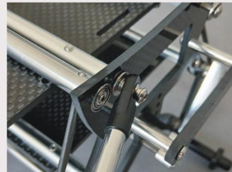
2) Attach the end of the lower links to the hole in the axle tubes you drilled earlier. Put the large washer over the screw, then put it through the axle tube from the outside. Add the 6mm spacer on the inside, then the lower link, and finally the rod end with sway bar attached.
