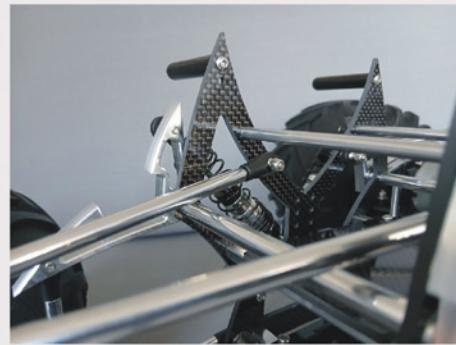
**3)** Attach the upper links to the middle hole on the gearbox top link mounts. With the 25mm screws and lock nuts.
