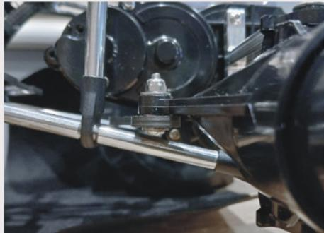
It's possible to swap the top link mounting points in the chassis with the alloy brace (shown in blue).
