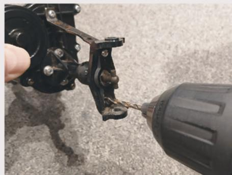
3) Fit the top link mounts to the gearboxes as shown, using the 6mm spacer at the rear and the cut washer at the front.
